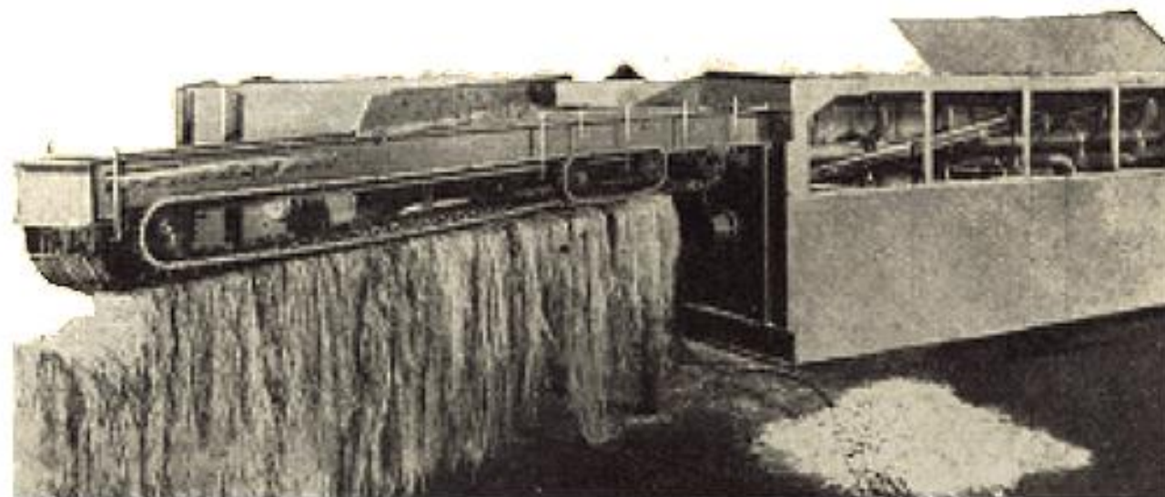
Hemp fiber being delivered from machine, ready for baling. Pile of pulverized hurds beside machine is 77 percent cellulose..
