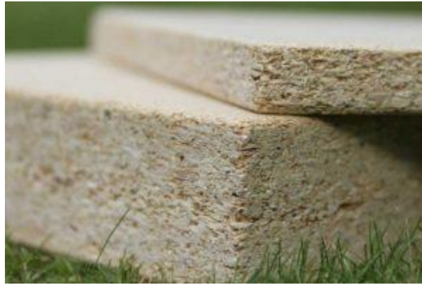
Figure 17. Particle boards from hemp as wood alternative in, for example, furniture production [138]
