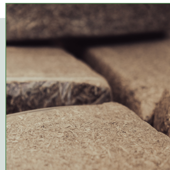
Processed hemp hurd bales ready for use in construction and insulation products
